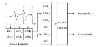
Fig. 1. Flow diagram of the proposed methodology with the details of the SQI features extracted (kSQI and sSQI) discussed in Section III.
