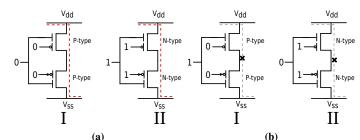
Fig. 10: Short-circuit and open-circuit configurations in RFETs-based inverters.
