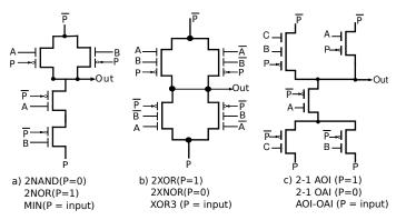
Fig. 7: Reconfigurable logic gates using RFETs [60]
