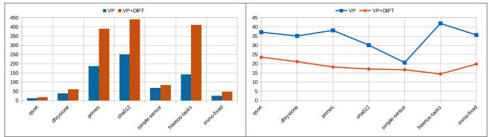
Fig. 4: Dynamic IFT performance overhead evaluation results - the left side shows the execution time in seconds and the right side the achieved MIPS for the normal VP (blue color) and the VP with dynamic IFT integration (orange color).
