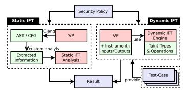
Fig. 3: VP-based static and dynamic IFT for security policy validation.
