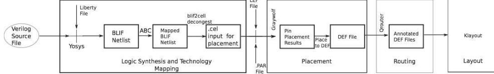
**Fig. 4:** Physical Synthesis Flow Through Qflow[13] Yosys [14] ABC[15] Graywolf[16] Qrouter[17] Klayout[18]
