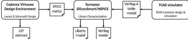
**Fig. 3.** Tool Flow for Library Characterization for Silicon Nanowires
