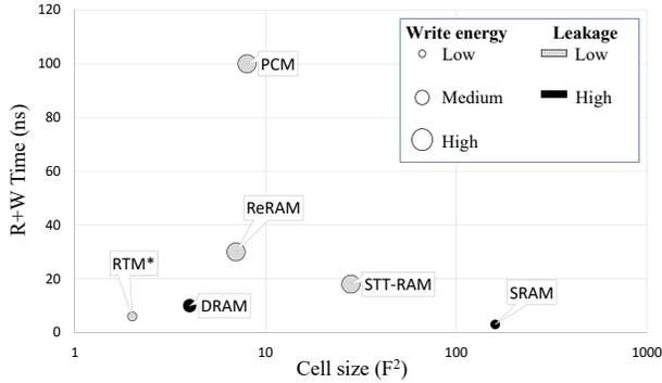
Fig. 2. Comparing different memory technologies (\*shift latency not accounted).
