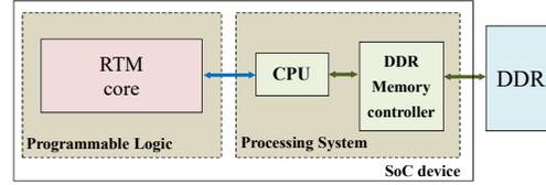
Fig. 6. Top-level architecture of ERMES.
