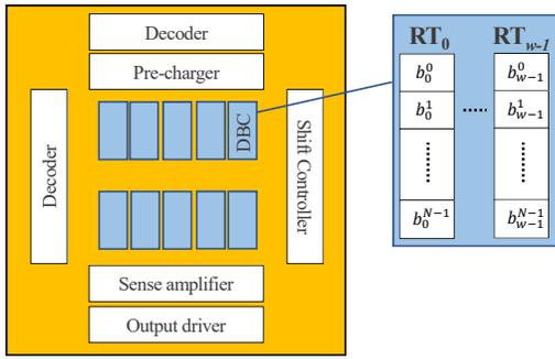
Fig. 5. RTM architecture.
