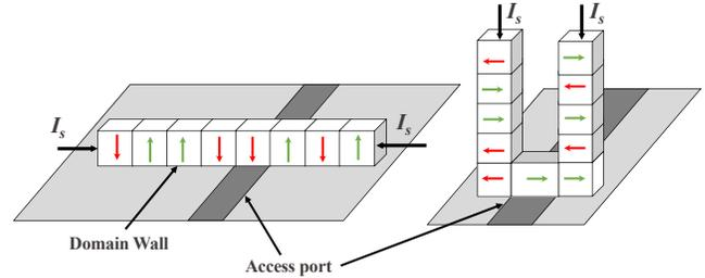
Fig. 3. Racetrack horizontal and vertical placement on a silicon wafer.
