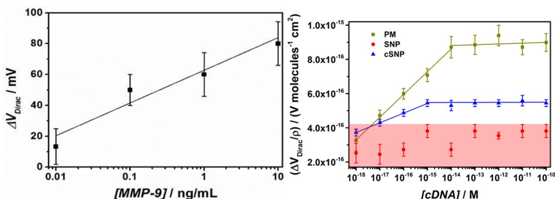
Figure 1: Calibration curves for A) an immuno-FET and, B) a DNA-FET. The curves are obtained by the average of five independent sensors, in order to obtain the error bars.
