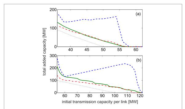
**Figure 5.** Comparison of strategies as in figure 4, but for random networks with an average degree of six (a) and four (b). We compare the three strategies defined in section 4: A: duplicating the critical line (blue dashed) B: adding a backup line of minimum capacity locally (red dash-dotted) C: adding capacity at bottlenecks nonlocally (solid green). The black dotted line shows the approximate lower bound (17).
