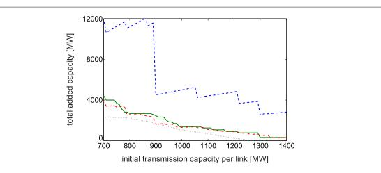
**Figure 4.** How much additional capacity is required to cure all critical links? We compare the three strategies defined in section 4: A: duplicating the critical line (blue dashed) B: adding a backup line of minimum capacity locally (red dash-dotted) C: adding capacity at bottlenecks nonlocally (solid green). The black dotted line shows the approximate lower bound (17). Results are shown for the test grid based on the topology of the Romanian power grid shown in figure 1.
