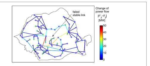
**Figure 3.** Response to the failure of a stable link. Fast drop off of the additional load with the distance from the removed link when the load has to be redistributed after the deletion of a stable link. The color codes the difference between the loads  $|F'_{j\ell'} - F_{j\ell'}|$  after and before the removal. It is pronounced only along the shortest alternative paths connecting the endpoints of the stable link.
