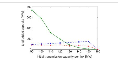
**Figure 6.** Comparison of strategies as in figure 4, but for a ring topology with one rewired link. We compare the three strategies defined in section 4: A: duplicating the critical line (blue dashed) B: adding a backup line of minimum capacity locally (red dash-dotted) C: adding capacity at bottlenecks nonlocally (solid green).
